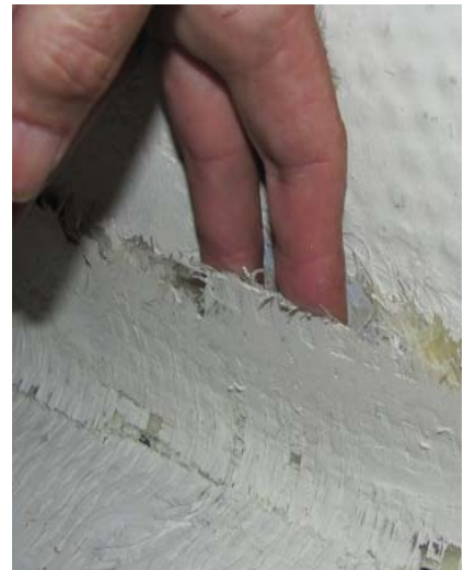
Interior separated bulkhead tabbing
