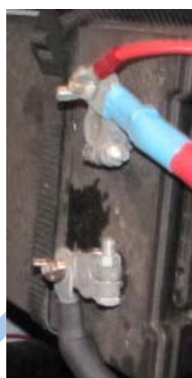
Loose wing nuts, unprotected positive terminals, unsecured batteries, low electrolyte
