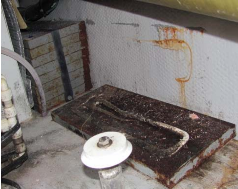
Approximately 367lbs. of unsecured and Inadequately secured ballast
