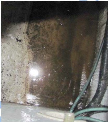
Various bilge compartments in engine room are heavily fouled
