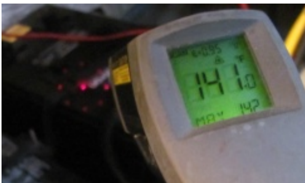
No. 5 battery at rest 141°F
