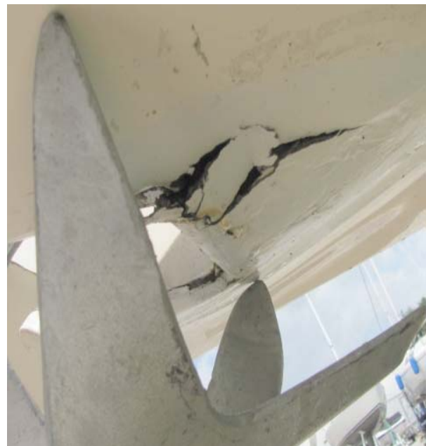
Underside bow platform fractured
