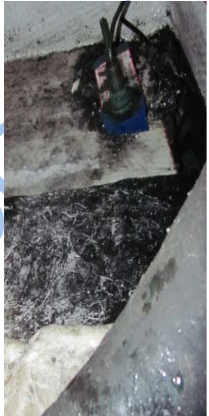
Various bilge compartments in engine room are heavily fouled
