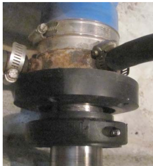
Port shaft - Stuffing retaining collar loose
