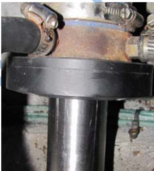
Starboard shaft – stuffing retaining collar missing
