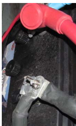
Loose wing nuts, unprotected positive terminals, unsecured batteries, low electrolyte
