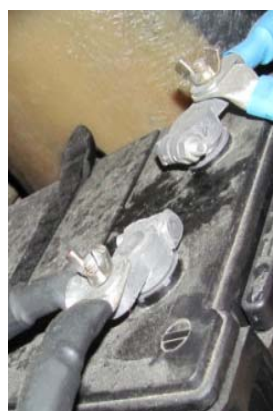
Loose wing nuts, unprotected positive terminals, unsecured batteries, low electrolyte
