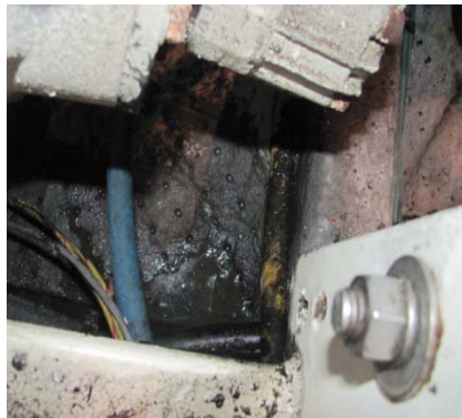
Various bilge compartments in engine room are heavily fouled
