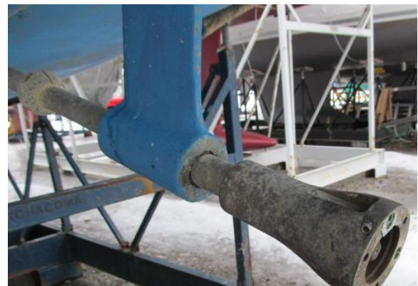
Feathering propeller, missing blades
