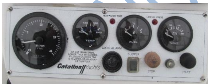
Tachometer stuck at 1000RPM
