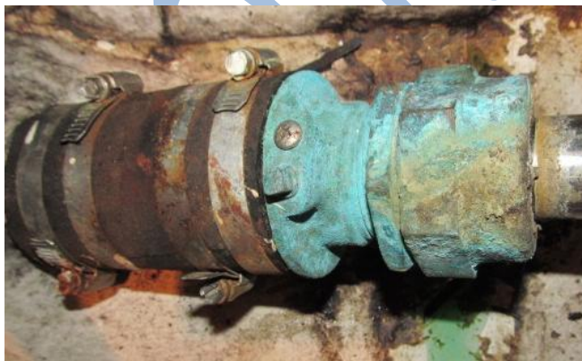
Corroded clamps and stuffing box
