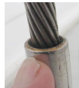
Port shrouds corrosion stains
