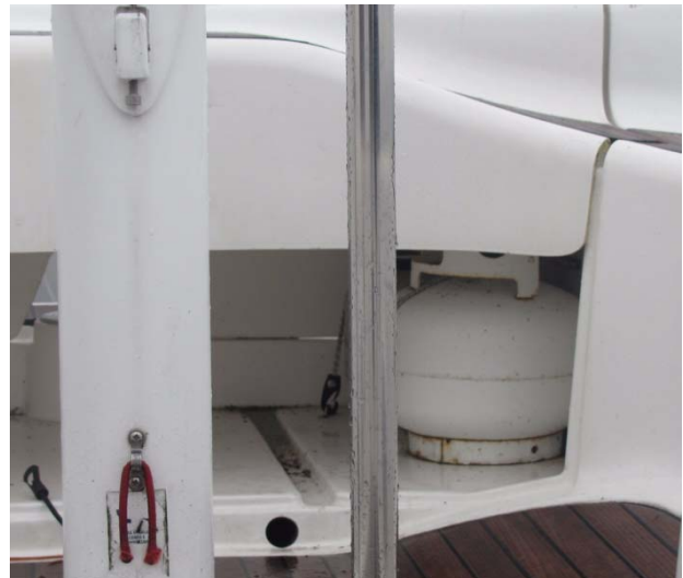
Propane bottle storage open to cockpit.
