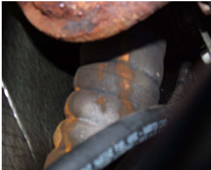
Brown sludge stains on exhaust hose below mixing elbow
