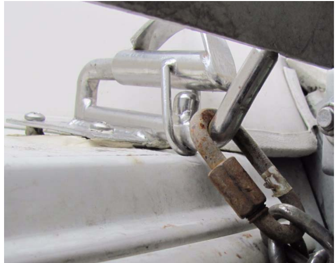
Weaver davit being used as a chain mount to support the dinghy platform and pulling free of deck.
