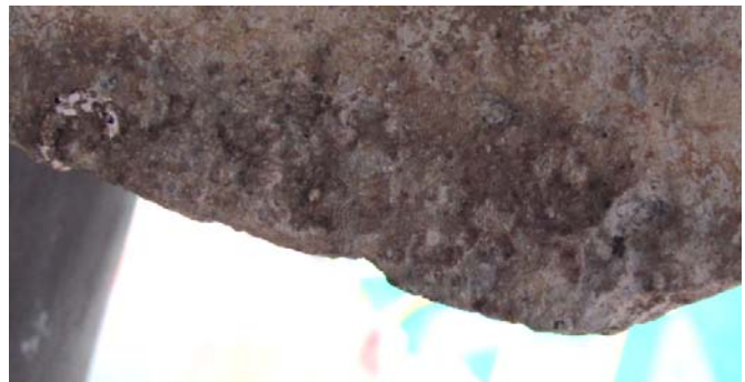
Corroded dinghy platform lifting arm.
